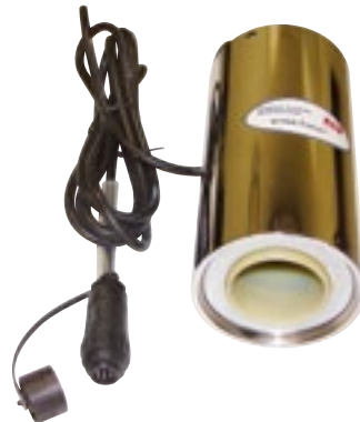
DYNA Force® Sensor for strand or bar
