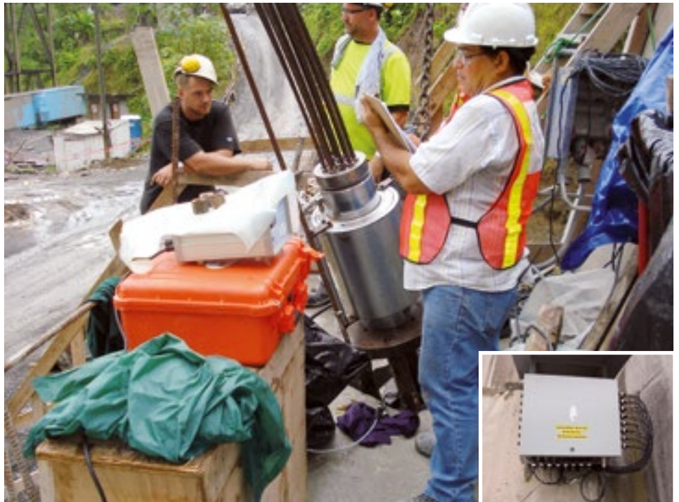
DYNA Force® for load monitoring of anchors at Changuinola Dam, Panama
